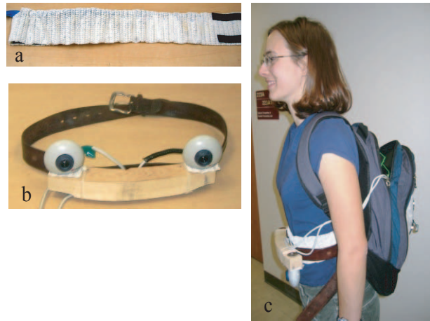
Fig. 1. Photograph of the navigation aid. a) The factor belt, containing 14 vibrating motors spaced laterally. b) The camera belt, with two webcams arranged to converge approximately 10 feet from the user. c) The full device from the side, as it is meant to be worn. Visual processing is performed by a laptop computer inside the backpack.
